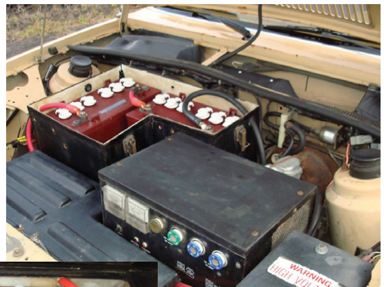
Above, front battery compartment and battery charger
