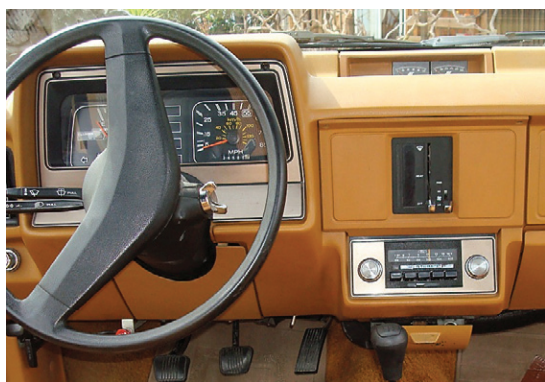
The small gauges at the top center indicate voltage and amperage.
