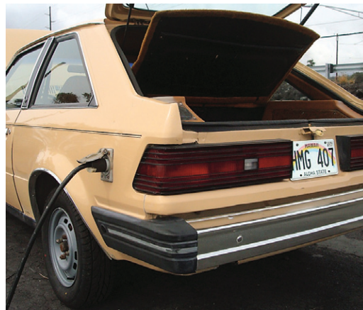
The 220 V electrical outlet. It can be plugged into a wall outlet or portable generator.
